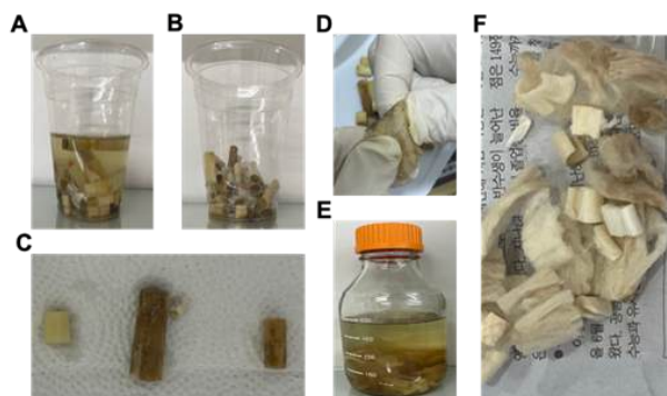
Figure 2. Clearance of cigarette butt filters (A, cigarette butt in water; B, cigarette butts with water removed; C, cigarette butt decomposition; D, separation of cigarette butt filters; E, filters in 70% ethanol; F, completely dried cigarette butt filters)
