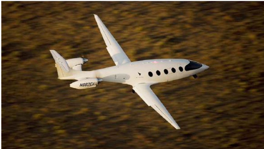
Figure 5. Alice – All-Electric Aircraft. This image shows the Eviation Alice, a fully electric regional aircraft designed for zero-emission flights. The aircraft features a sleek fuselage, low-wing configuration, and twin aft-mounted propellers, optimizing energy efficiency and aerodynamic performance. (Eviation Alice, 2025).
